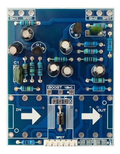
Solder the capacitors and transistors. If you have troubles reading the values, check out our <u>"Reading Part Values"</u> tutorial. Pay attention to the orientation, as well as to the polarity for electrolytic capacitors.
