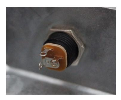
Then, solder the three wires from the DC connector in the board to the DC jack as follows:
